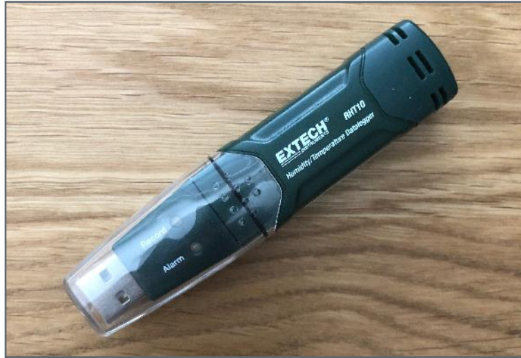
Image 10: Extech RHT10 data loggers used to record conditions in the Great Room as well as ambient conditions outside the building.
