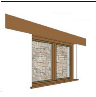
A. Exposed Timber Lintel
